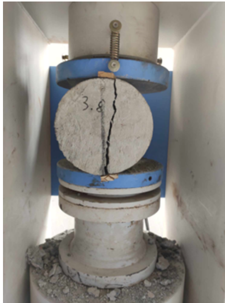
FIGURE 8. Split Tensile Strength Test Specimens.
