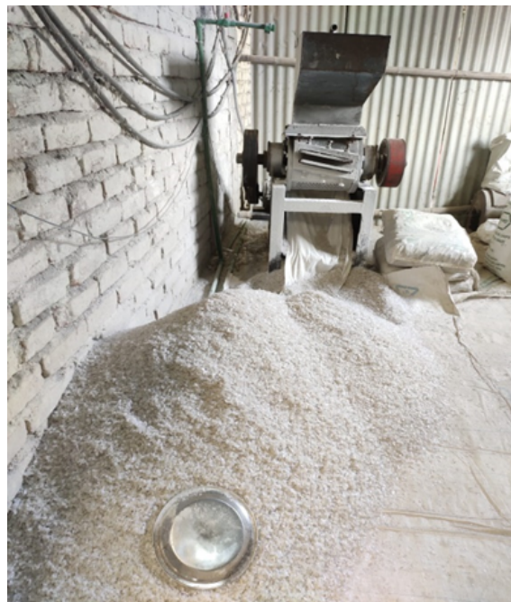
FIGURE 2. Shredding Machine for Powdered PET.
