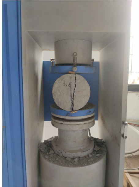
FIGURE 6. Failure Modes of Specimens.
