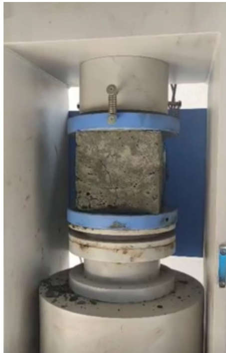
FIGURE 5. Preparation of Compression Test Specimens.
